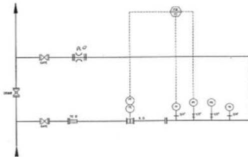
There are two ways to install a Master Meter on an existing Field Meter skid. One way is to use a three-valve manifold downstream of the existing meter run shown in the P&ID above. Downstream of the field meter is the preferred location because the flow profile into the Field Meter is not disturbed.
