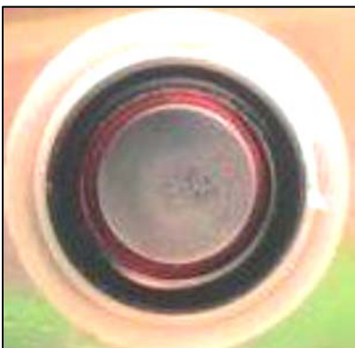
Figure 1. Gas at the Hydrocarbon Dew Point in a Chilled Mirror Device
