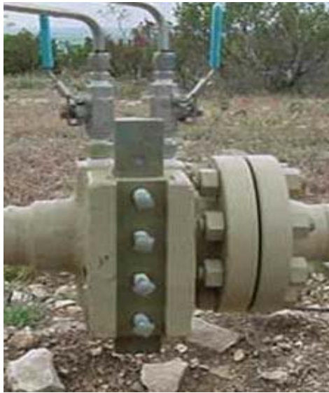
Figure 5. Single chamber fitting with flange tap valves
