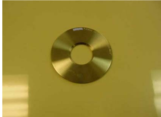
Figure 3. A universal orifice plate.
