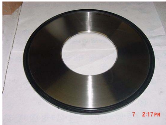
Figure 4. A universal plate with seal ring.
