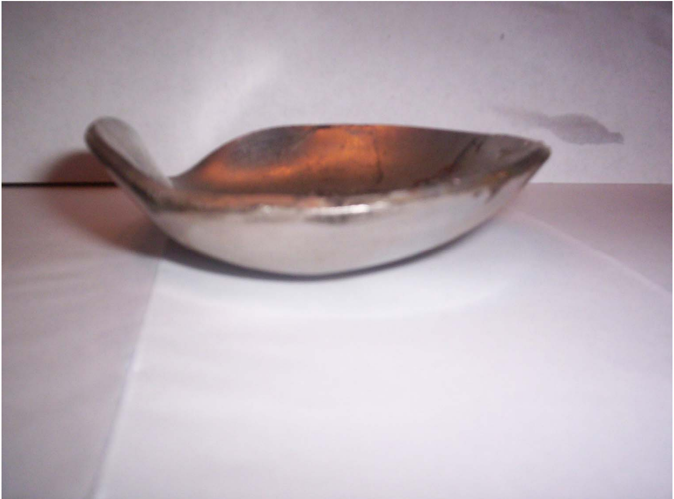
FIGURE 4. Orifice Plate Damaged by Loose Straightening Vanes
