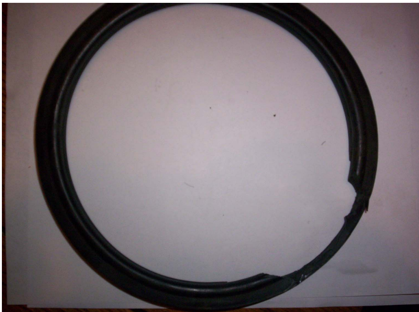
FIGURE 5. Torn Seal Ring
