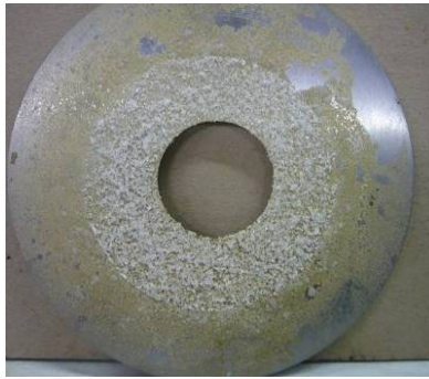
Fig 21. A heavily contaminated orifice plate
