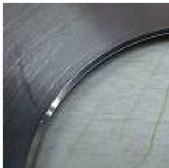
Fig 18. Chamfered (0.02") orifice edge
