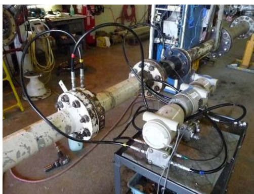
Fig 5. Flange installed plate with air flow
