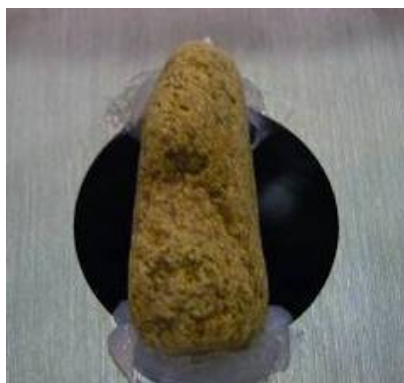
Fig 29. Rock trapped at an orifice plate
