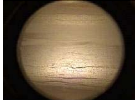
Fig 26. CEESI wet gas view port of wet gas flow upstream of orifice meter
