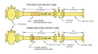
Figure 5 – Meter Tube with Strainer and Flow Conditioning
