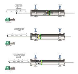
Figure 11 – Typical Prover Operation
