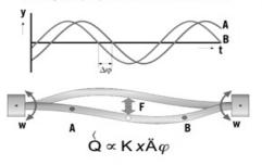
Figure 9 – Schematic of Coriolis Meter Guiding Principals
