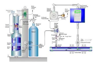
Figure 13 – Typical NGL Sampler Setup
