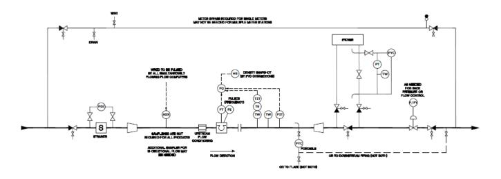
Figure 14 - Direct Mass Measurement Skid
