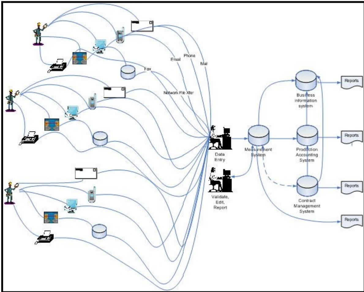
Figure 3. Manual Field Data Capture - Data Flow
