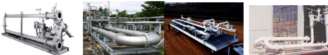
Figure 5. Different Ball Prover Configurations
