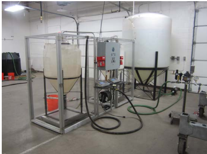
Figure 3. ISO 17025 Certified Gravimetric Water Draw Test Stand – Flow MD – Phoenix, AZ
