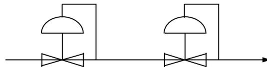
**FIGURE 4. Series Regulation Schematic**
