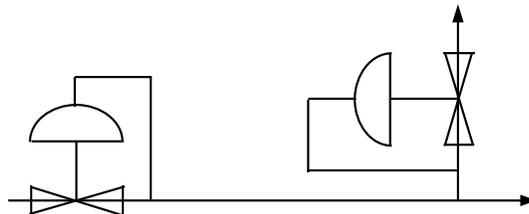
**FIGURE 1. Relief Schematic**
