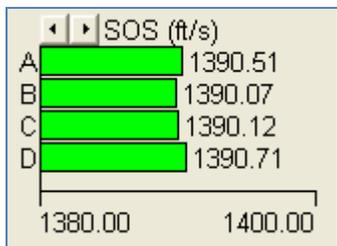
It is worth chasing the error down as mis-measurement of temperature has a significant effect on the standard volume measurement (the ultrasonic meter is measuring actual volumetric flow and is unaffected by gas pressure, temperature or gas composition). Temperature in error by 1° F in the previous example will cause the corrected volumetric calculation to be incorrect by 0.28%. Using a calculated speed of sound vs. measured is a great check of a stations' temperature measurement.
