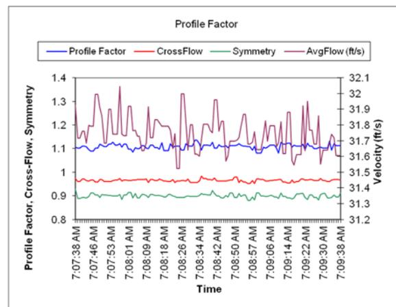
This could indicate a blockage upstream of the meter.
